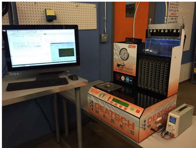
*Proper characterization data cannot be accurately obtained unless proper equipment is used and proper procedures are followed. DW's in-house process was developed using SAE J1832. Accuracy is obtained by using temperature controlled calibration fluid, NIST traceable pressure gauges, highly sensitive digital flow meters, and fully adjustable digital injector drivers with proper fly back loops.*
